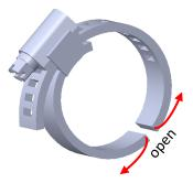
Clamp B has the cut on the opposite side the adjusting unit. Gently spread the clamp and push it over the hose.
