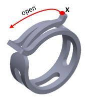
After removing all supports one grab the end of the clamp marked as X and gently pull it in order to adjust clamp diameter or to make it fully open. In case the one has fully withdrawn end X from the clamp, it can inserted inside the clamp again to recreate the original shape.
