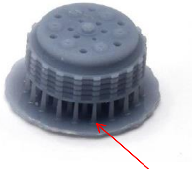
Supports to remove
