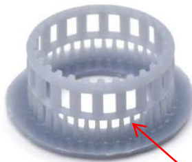
Supports to remove
