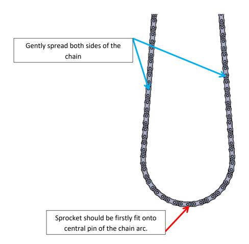
Proper position of the sprocket inside the chain (general view).
