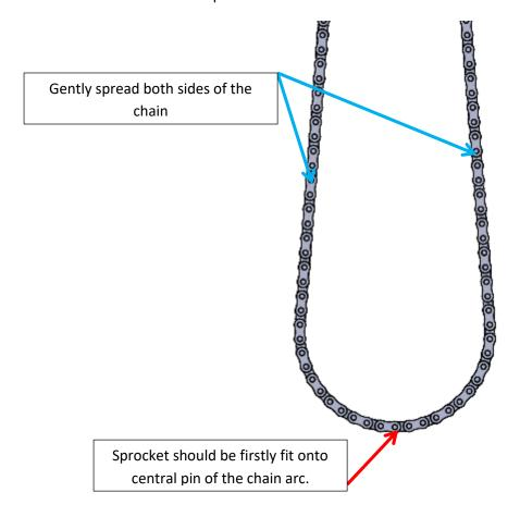
Proper position of the sprocket inside the chain.
