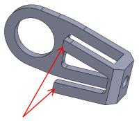
Inner elements must touch the cylinder on which you will install the B30.
