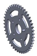
4. In the rear sprocket adapter (7) correct holes diameters with 1mm drill. Apply small amount of CA glue inside the screw holes in the adapter and joint it with installation pins of screws joined with the rear sprocket.
